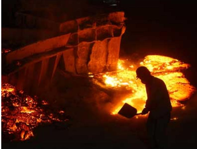
The more advanced way to smelt iron is in a blast furnace. A blast furnace is charged with iron ore, charcoal or coke (coke is charcoal made from coal) and limestone ( $\text{CaCO}_3$ ). Huge quantities of air blast in at the bottom of the furnace, and the calcium in the limestone combines with the silicates to form slag. Liquid iron collects at the bottom of the blast furnace, underneath a layer of slag. The blacksmith periodically lets the liquid iron flow out and cool.
